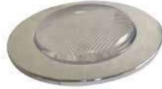
SR13296 Gömme Spot Krome 12V 15 Led SR13298 Gömme Spot Krome 24V 15 Led Çap: 92 mm, Montaj Çapı: 75,5 mm, Derinlik: 12 mm
